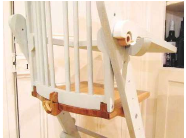
◀ Pic.6 The legs, which fold flat, are braced with thin struts and stop-bars. The struts are held together with halving joints, and pegged and glued to the legs
